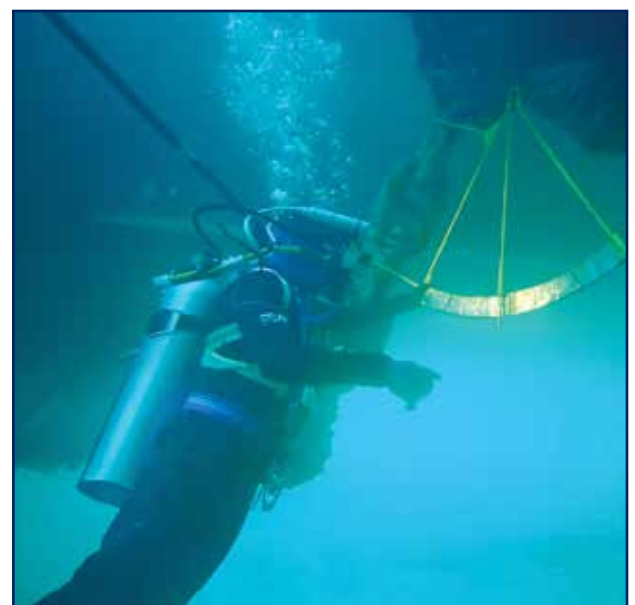
Professional Diving Services - Chain Angle Measurement
