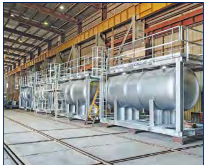
Gas Scrubber Package for Joint Operations - Wafra
