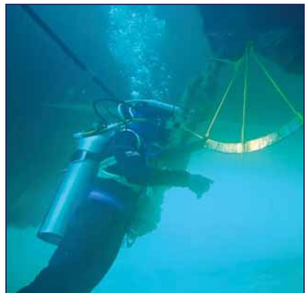
Professional Diving Services - Chain Angle Measurement
